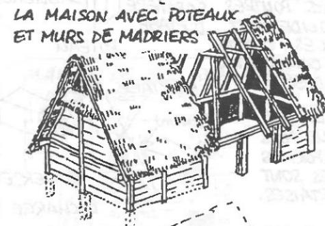
LES POTEAUX SONT ENTERRES, ET AU BESOIN CONSOLIDES INDIVIDUELLEMENT A L'AIDE DE BOIS FORMANT DES SEMELLES D'APPUI. ENTRE LES POTEAUX, LES MURS SONT COMPLETES AU MOYEN DE MADRIERS REPOSANT LES UNS SUR LES AUTRES.
